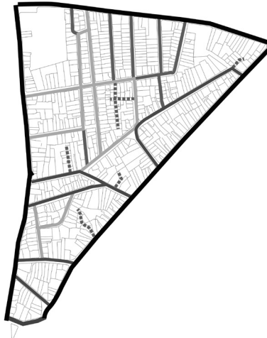
Evolution of the road layout. From black to light grey: matrix routes, connecting route, back routes, arteries that appeared between 1911-1974. Unfinished back routes are marked with dotted lines.
